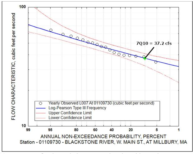
Figure 2: Log-Pearson fit to the Annual 7-day Average Low-Flow Values and the 7Q10 Flow at USGS Gage 01109730 at Millbury
