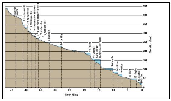
Figure 1: River elevation profile
