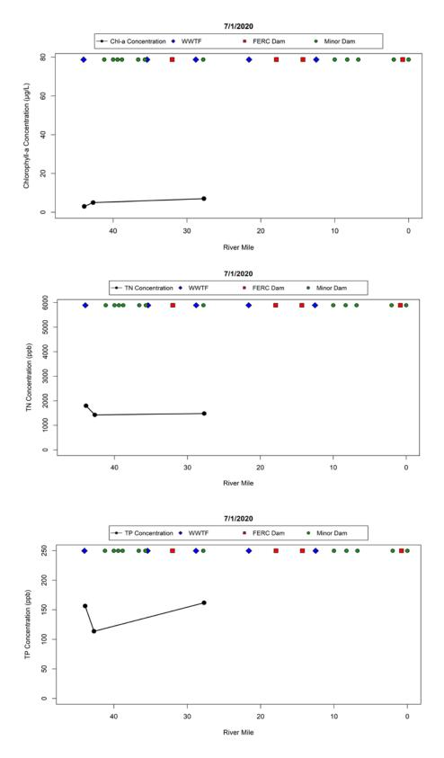
Figure B4: July 1 (treated as June) 2020 along stream concentration (Chl-a, TN, TP)
