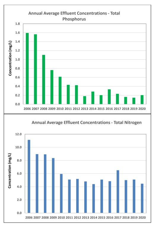
Figure 14: Annual average effluent total phosphorus and total nitrogen concentrations 2006 – 2020
