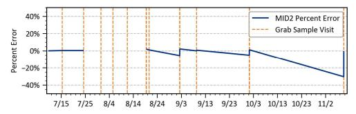
Figure 6: Percent Error at MID2 between the In Situ Meter and the Handheld Field Meter
