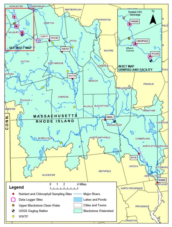
Figure 1: Upper Blackstone Sampling Locations: 2020 Continuous Dissolved Oxygen Meters Installed at W0680, UBWPAD2, W1258, and MID2 (Depot)
