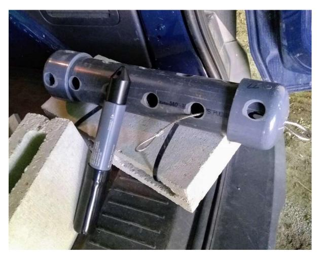
Figure 4: Dissolved Oxygen Meter Housing and Cinder Block Anchor
