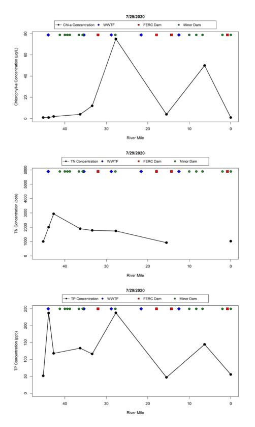
Figure B5: July 29 (treated as July) 2020 along stream concentration (Chl-a, TN, TP)
