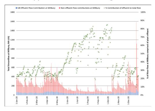
Figure B1: Effluent flow contributions at Millbury, 2020
