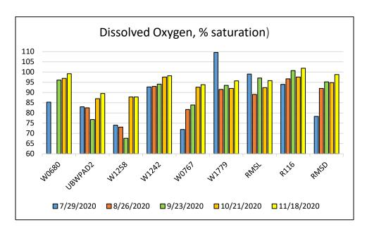
Figure 45: 2020 Dissolved Oxygen Percent Saturation at each site
