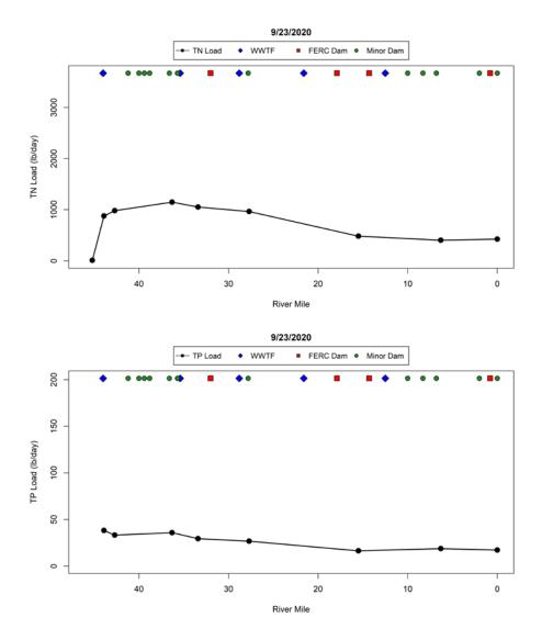
Figure B13: September 2020 along stream load plots (TN, TP)
