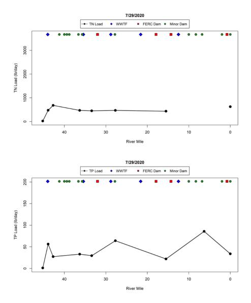
Figure B11: July 29 (treated as July) 2020 along stream load plots (TN, TP)
